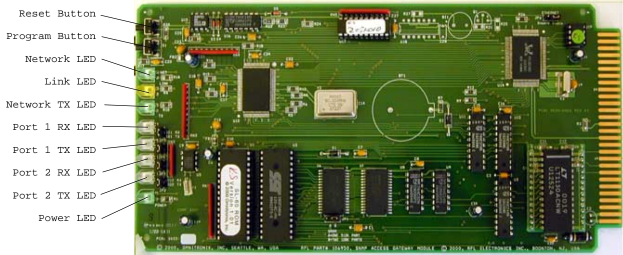
Figure 5. – SNMP Access Gateway Module Layout
