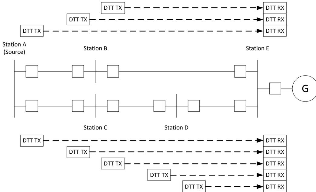
**FIGURE 3: LOOPED SYSTEM ANTI-ISLANDING WITH PHASE COMPARISON**
