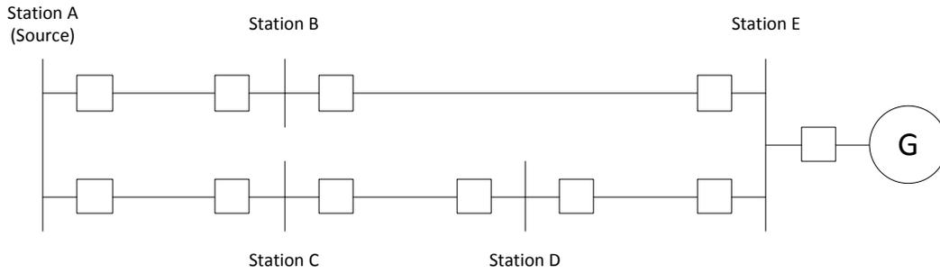
**FIGURE 2: LOOPED SYSTEM ANTI-ISLANDING WITH DTT**
