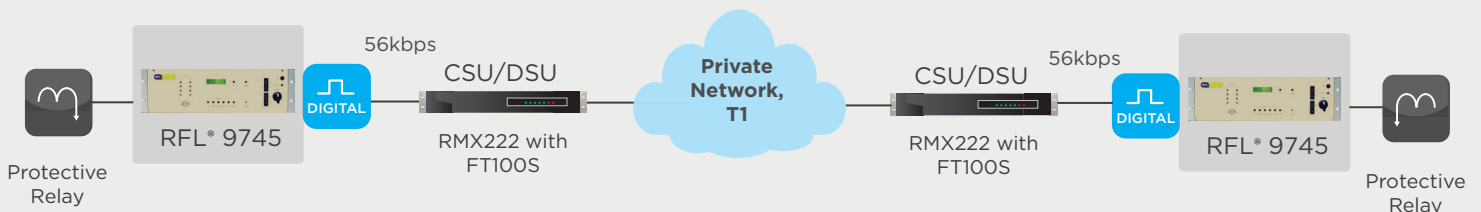
After Upgrade: Digital Teleprotection over T1 leased lines
