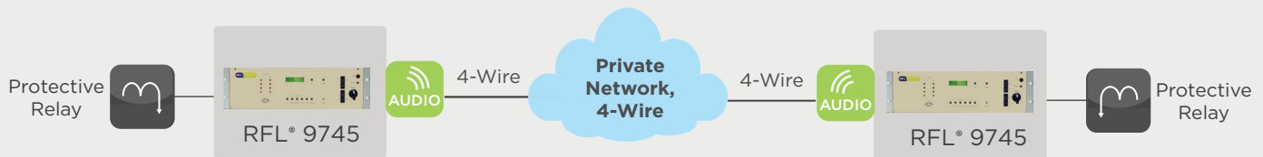
Before Upgrade: Analog Teleprotection over 4-wire leased lines
