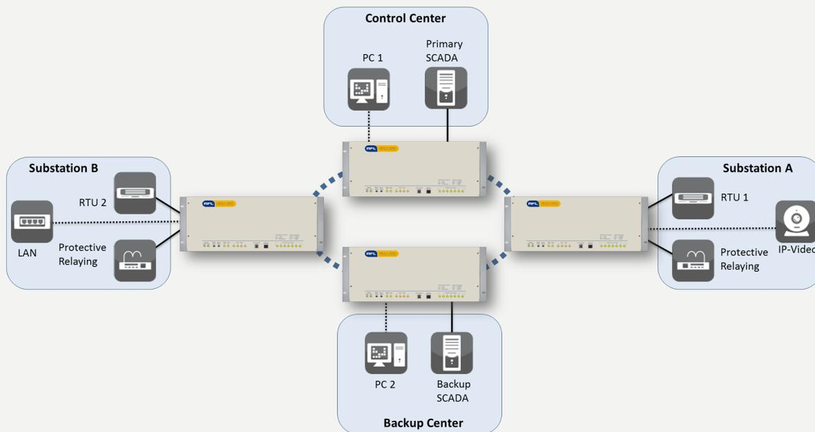
**Figure 2: Gigabit Ethernet Ring network carrying legacy SCADA/RTU, Protective Relaying and IP-based services**
