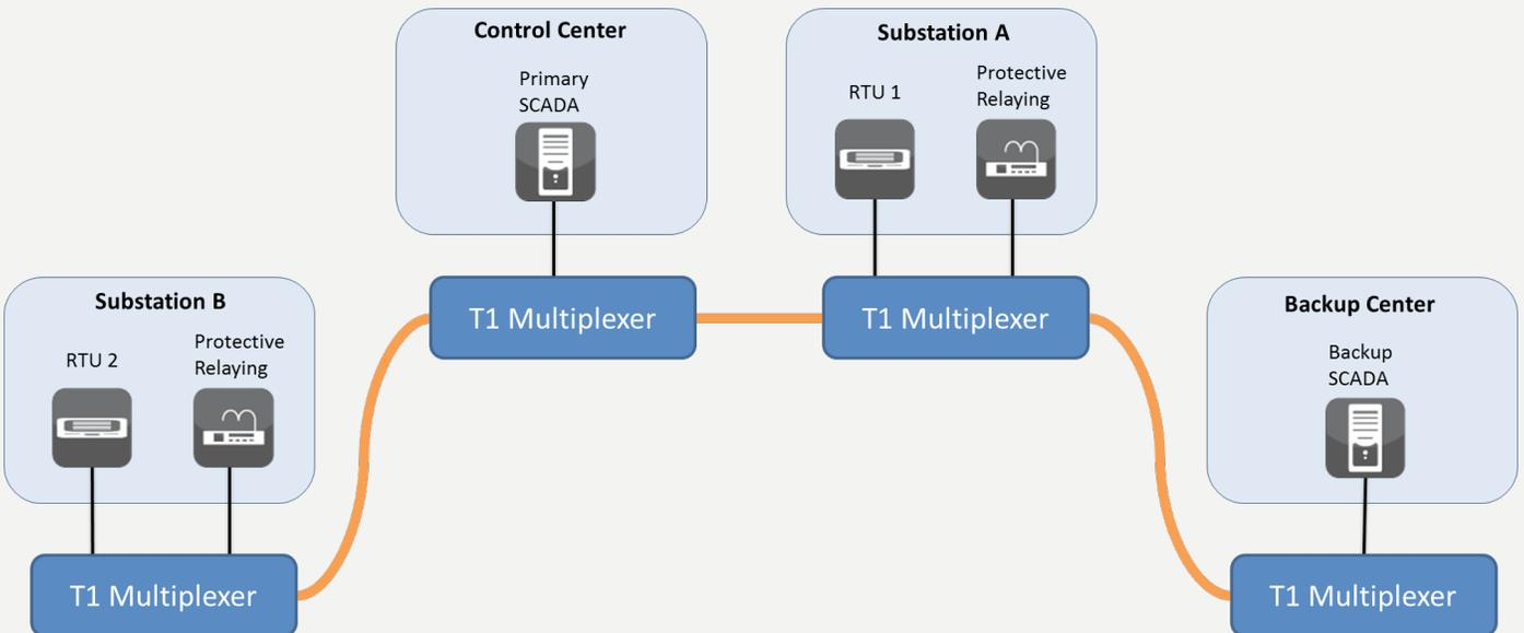
**Figure 1: Linear Add/Drop T1 network carrying SCADA/RTU and Protective Relaying**
