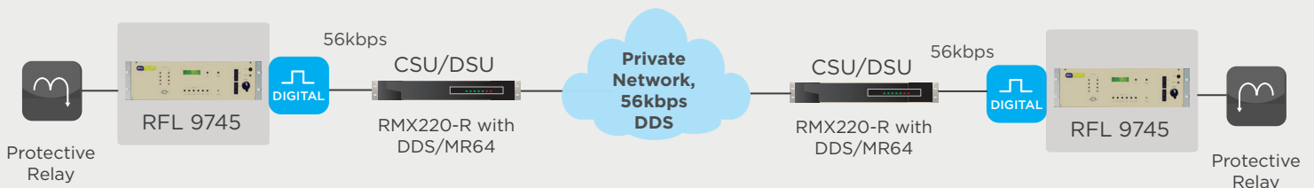
After Upgrade: Digital Teleprotection over DDS leased lines
