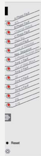
Figure 3. GARD 8000 Front Panel LEDs (6U)
