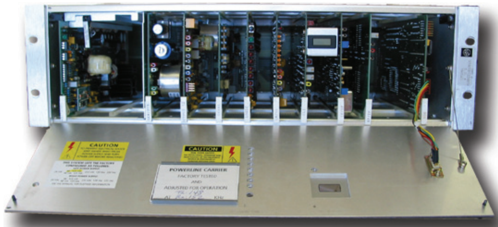
Figure 4. Typical RFL® 9780 Programmable FSK Power-Line Carrier Front Panel Down.
