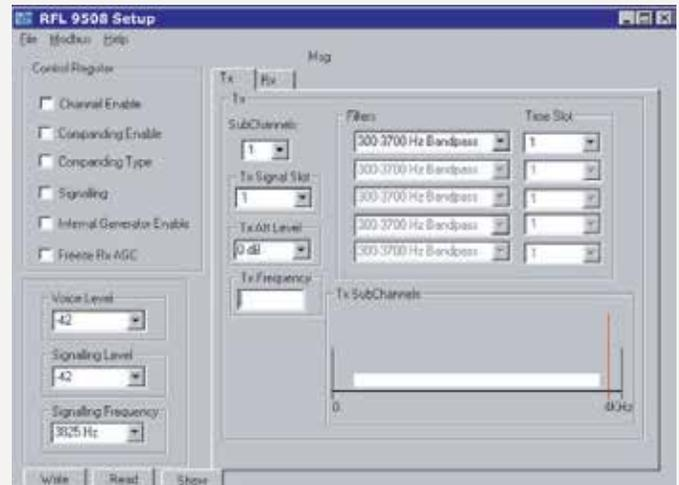
Figure 2. Typical Setup Screen
