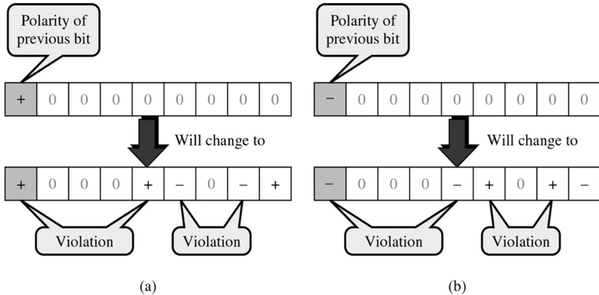
Figure 7. Bi-polar with 8-zero substitution (B8ZS)
