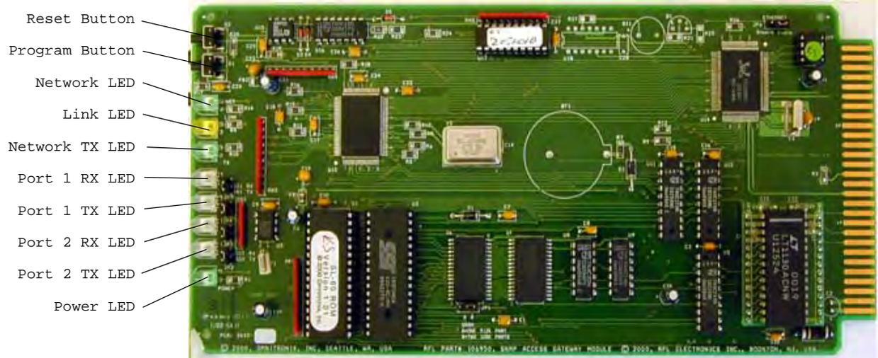
Figure 5. – SNMP Access Gateway Module Layout
